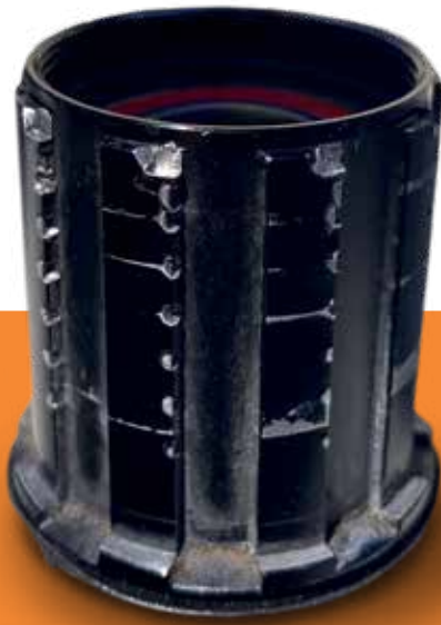
Damaged Aluminum Freehub Body
